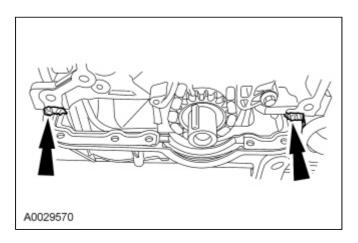
4. Apply silicone gasket and sealant to the front cover in 2 places.
