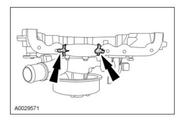
5. **NOTE:** Apply thread sealant to the stud bolts and make sure that the stud bolts are installed in their original positions.
